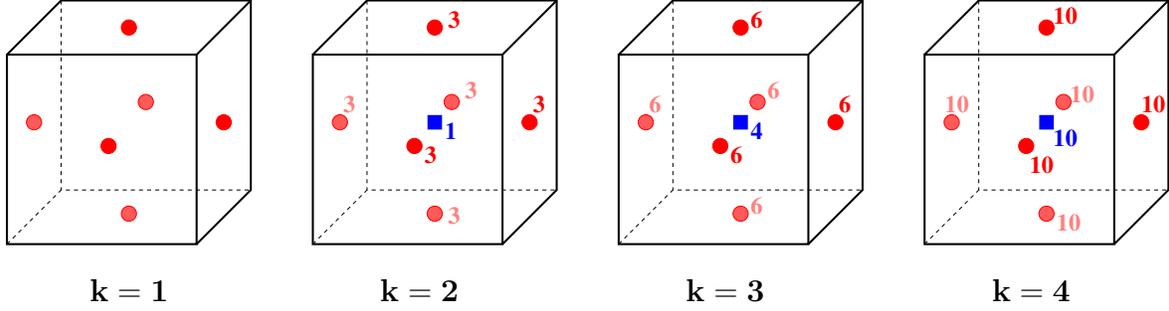
Figure 3.5. Degrees of freedom of a cubic cell for  $k = 1, 2, 3, 4$ ; face moments are marked by a circle; cell moments are marked by a square. The numbers indicate the number of degrees of freedom (1 is not marked in the plot for  $k = 1$ ).
