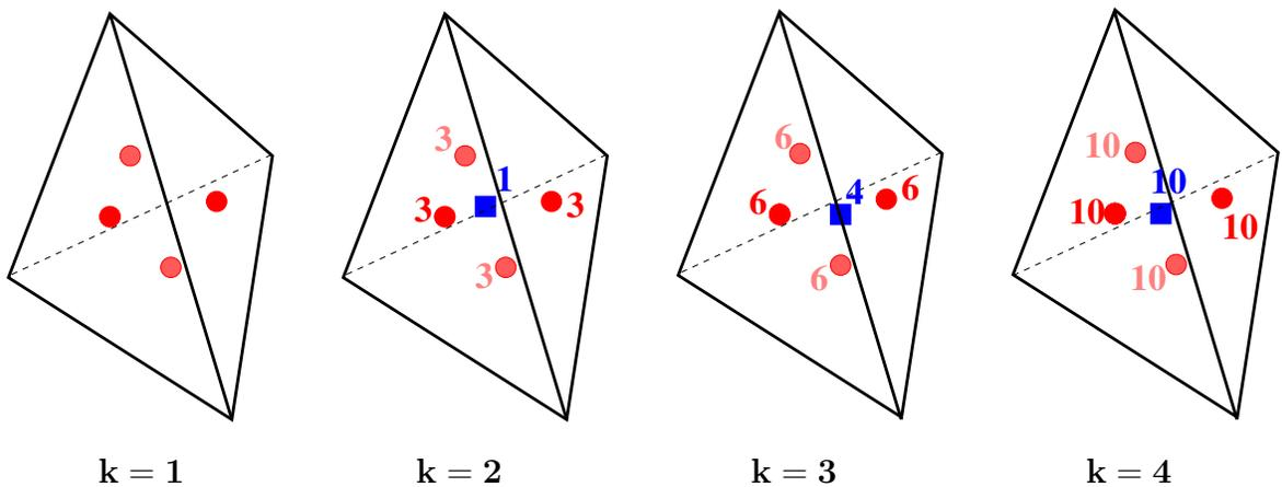
Figure 3.4. Degrees of freedom of a tetrahedral cell for  $k = 1, 2, 3, 4$ ; face moments are marked by a circle; cell moments are marked by a square. The numbers indicates the number of degrees of freedom (1 is not marked in the plot for  $k = 1$ ).
